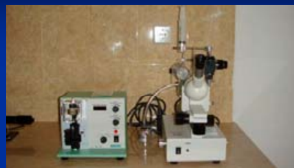
Grinder unit to make micro needle
