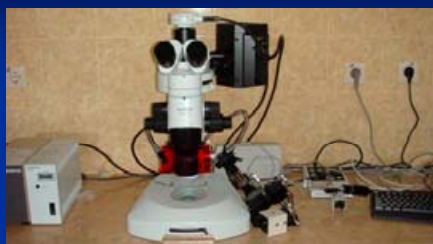
Microscope and equipments for gene transfer by microinjection and detect GFP expression
