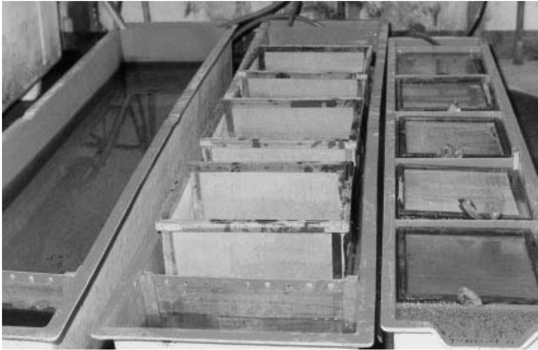
Fig. 2 - Incubation trays made of screen and placed in fiberglass incubation apparatus
