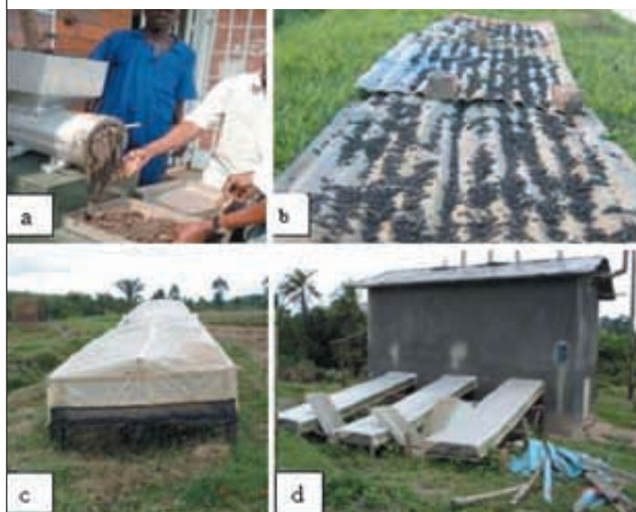
FIGURE 5 Feed processing and drying (a) feed pelletter (b) direct sun drying on corrugated iron sheet (c) solar dryer (d) improved solar dryer
