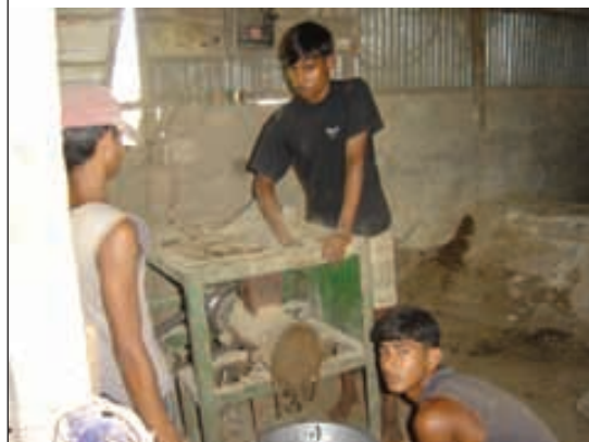
FIGURE 5 Workers involved in making pellets in a small-scale fish feed mill at Narshindi Sadar, Narshindi, Bangladesh
