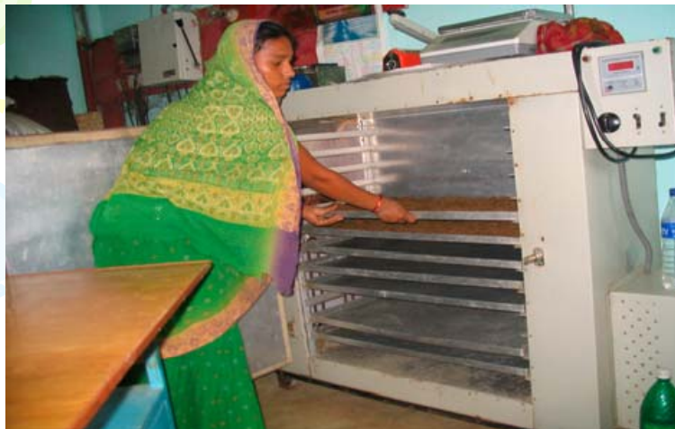
Drying of the Feeds by Mechanical dryer
