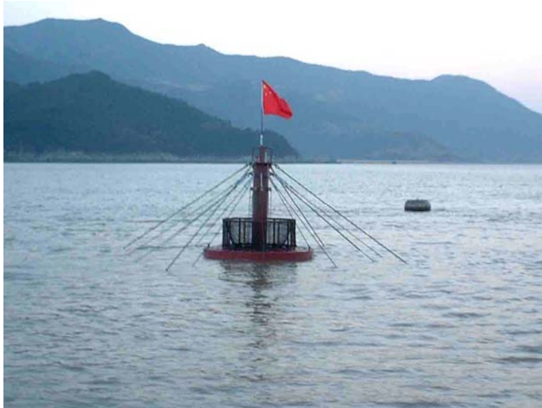
Fig 7 Dish-formed cage (made in Zhejiang Province)
