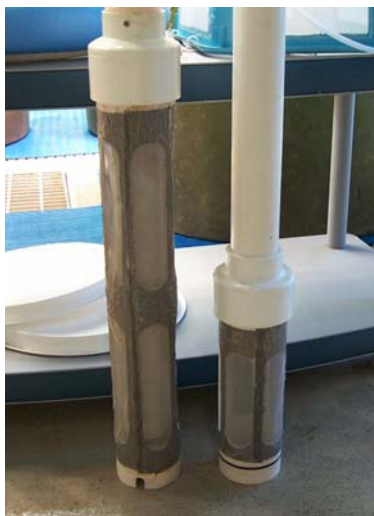
Figure 18 (left) Centre airlifts with stainless steel screens (105 \mu\text{m} ) to exclude copepodids and adults.
