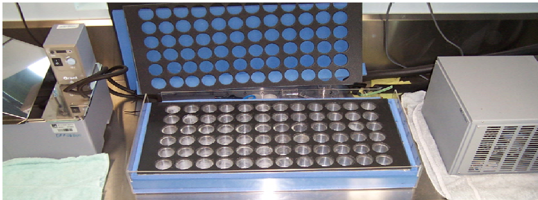
Figure 21 Temperature gradient block consisting of 12 columns (12 temperatures) and 6 rows (6 replicate temperatures). Refrigerated and heated water baths are attached to opposite ends of the block.
