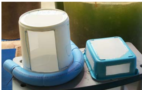
Figure 19 (below) Floating, screened (53 \mu\text{m} ) egg-nauplii collection vessels.
