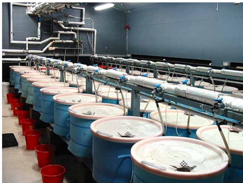
Flow-through constant temperature seawater experimental array consisting of 48 x 100 L insulated tanks at CSIRO used for grouper nutrition research.
