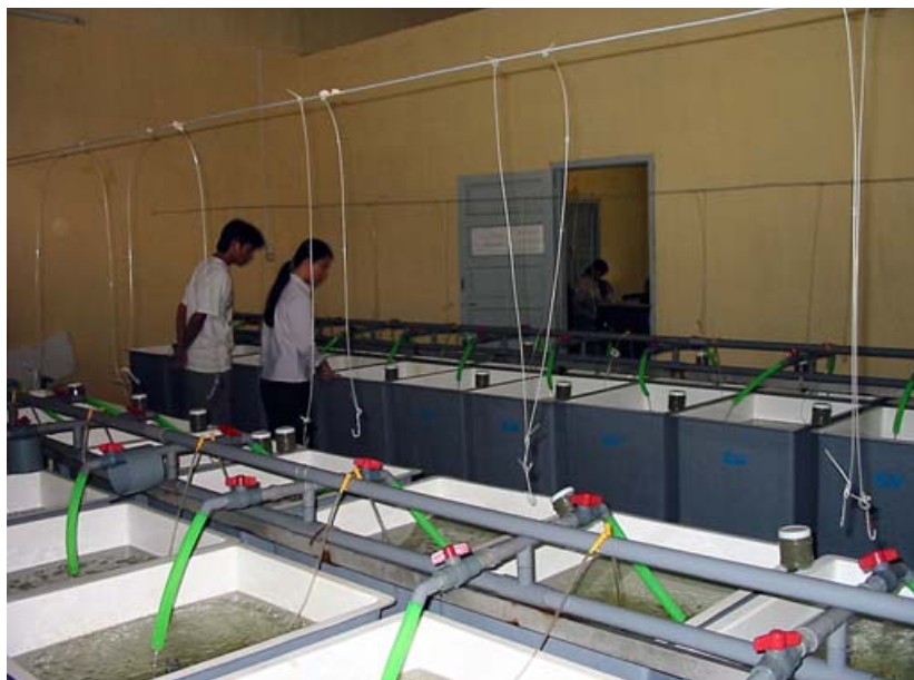
University of Fisheries' nutritional wet laboratory comprising 48 experimental tanks.
