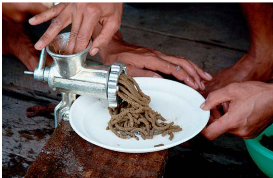
Preparation of moist feed pellets (noodles) using simple on-farm equipment. A kitchen meat mincer is used to mince the trash fish. The mixed dough is extruded through the meat mincer and the resultant noodles subsequently broken into suitable lengths for feeding to groupers.
