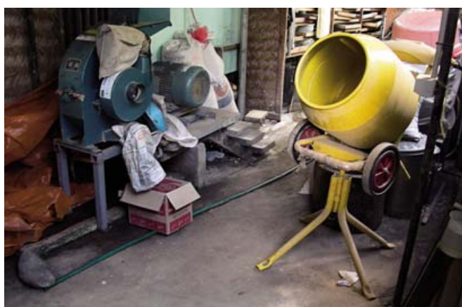
A pelleted feed ingredient grinder (left) and an ingredient mixer (right) at a small-scale feed making centre.
