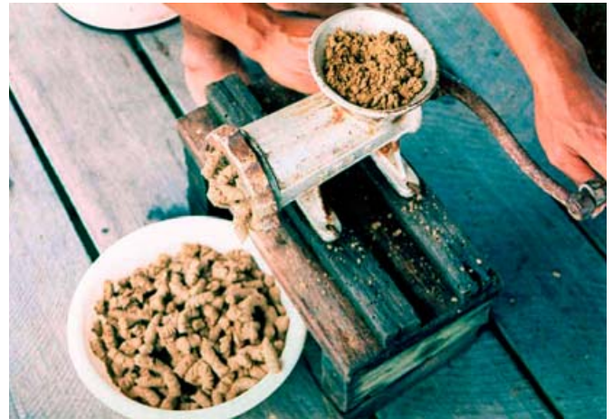
Figure 3. Manual preparation of noodle (pellet strands) by cold extrusion.
