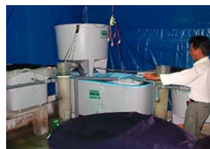
Mr. Thach Thanh explaining his recirculating broodstock maturation system with on the left the individual broodstock containers and in the middle the filter unit with "homemade" protein skimmers and the submerged and trickling filter.
