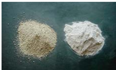
Fig. 1. A finely-ground agricultural limestone (right) versus a coarsely-ground one (left).
