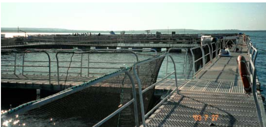
Sea cages used at Marine Harvest's Tiwi Island (near Darwin) barramundi farm, which produces about 1,500 tonnes of fish per year. Problems with crocodile and shark predation has been overcome using stainless steel mesh.
