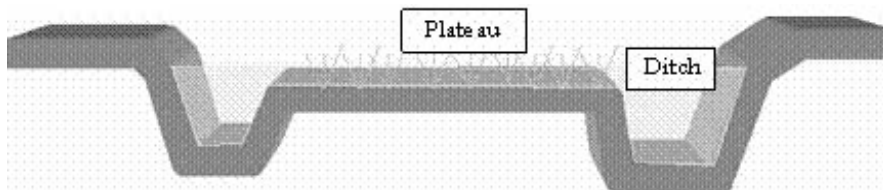
Figure 1: Section of the rice-shrimp farming system.
